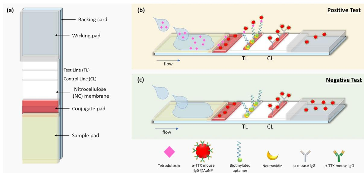
**Figure 1.** Schematic illustration of the TTX LFA tests. Design of the strips (a) and representation of the detection process in the presence (b) and absence (c) of TTX.
