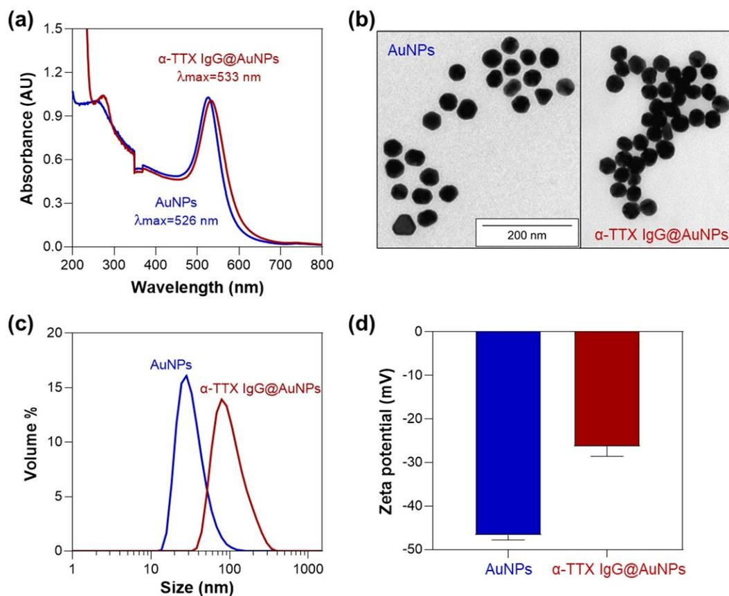
**Figure 2.** Characterization of the  $\alpha$ -TTX IgG@AuNPs conjugate by (a) UV-Vis spectroscopy, (b) TEM, (c) DLS and (d) Zeta potential measurements.
