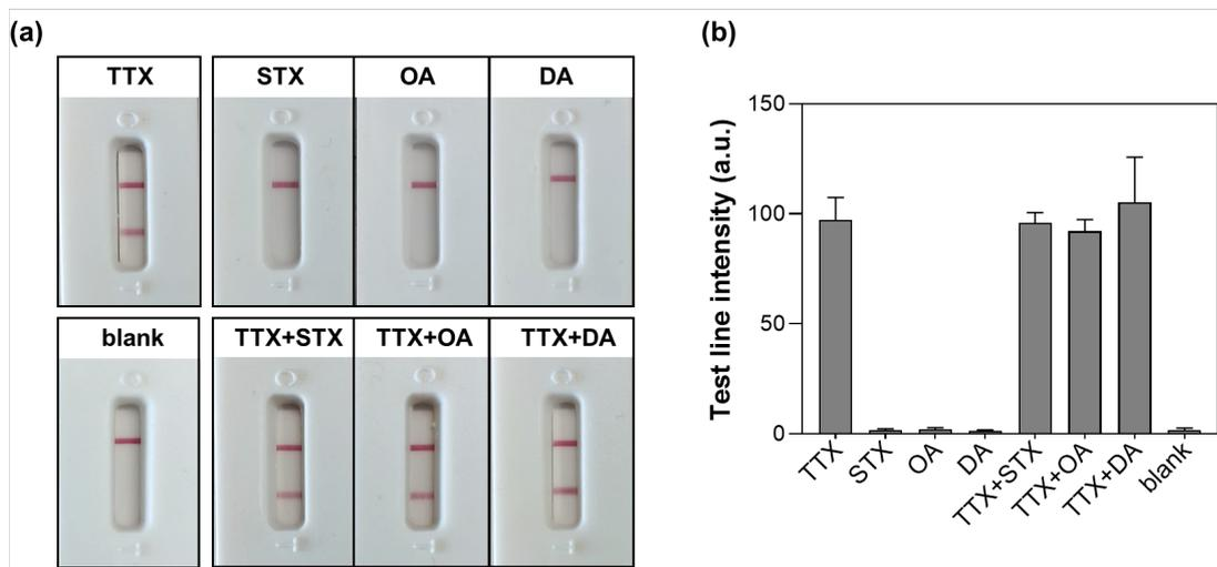
**Figure 5.** Specificity of the LFA test. TTX (1 ng/mL) or other marine toxins (20 ng/mL) were analyzed with the tests, individually or in mixtures. (a) Representative images of the LFA tests. (b) Quantification of the tests with the Cube LFA reader. STX: saxitoxin; OA: okadaic acid; DA: domoic acid;  $n=2$ , error bars:  $\pm$  SD.
