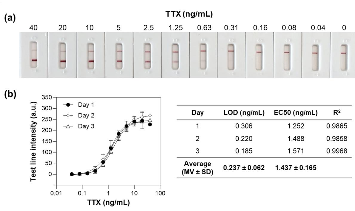
**Figure 4.** Sensitivity and reproducibility of the LFA tests. (a) Representative images of the tests where TTX standard solutions of 0.04 – 40 ng/mL were analyzed. (b) Calibration curves constructed after measuring the test line intensities with the LFA reader. Three independent experiments were performed with duplicate measurements.
