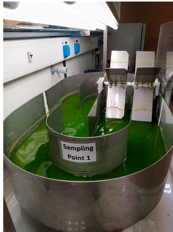
Figure 1. Cultures of selected microalgae in an open raceway pond photobioreactor (ORWP) ( V_w = 40 L). The photobioreactor has the following dimensions: an outside length of 110.5 cm and an inside length of 80 cm, with a width of 61 cm. Its total depth is 20 cm, while the culture depth specifically measured 7.5 cm. Culture conditions: modified artificial seawater (mASW), pH: 8.5, temperature: 23 \pm 1 °C, photoperiod: 24:0, light intensity: 27\text{--}34 \mu\text{E}/(\text{m}^2 \cdot \text{s}) , agitation: 35 rpm by using a double 4-bladed paddlewheel.
